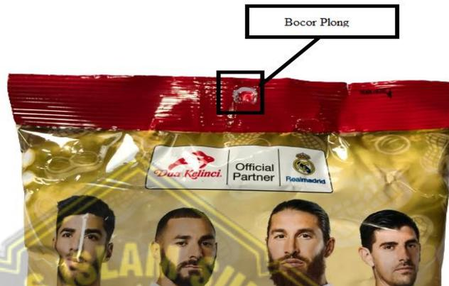
**Gambar 4.4** Bocor Plong
