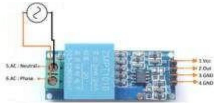
**Gambar 2.12** Sensor Tegangan ZMPT101B [27]
