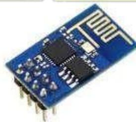
**Gambar 2.14** Modul ESP8266-01 [29]
