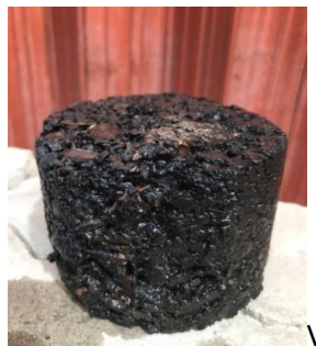
Gambar 3.27 Hasil perendaman 12 jam air lab
