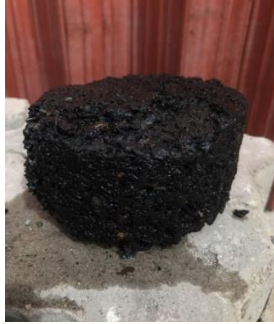
Gambar 3.25 Hasil perendaman 48 jam air lab
