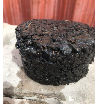
Gambar 3.26 Hasil perendaman 48 jam air lab
