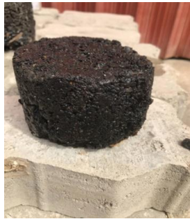
Gambar 3.19 Hasil perendaman 6 jam air lab
