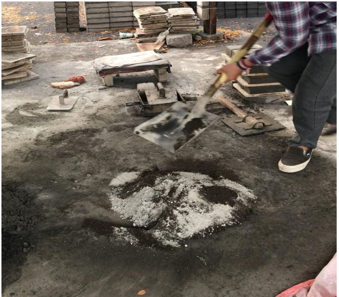
Gambar 7. Pengadukan campuran paving block
