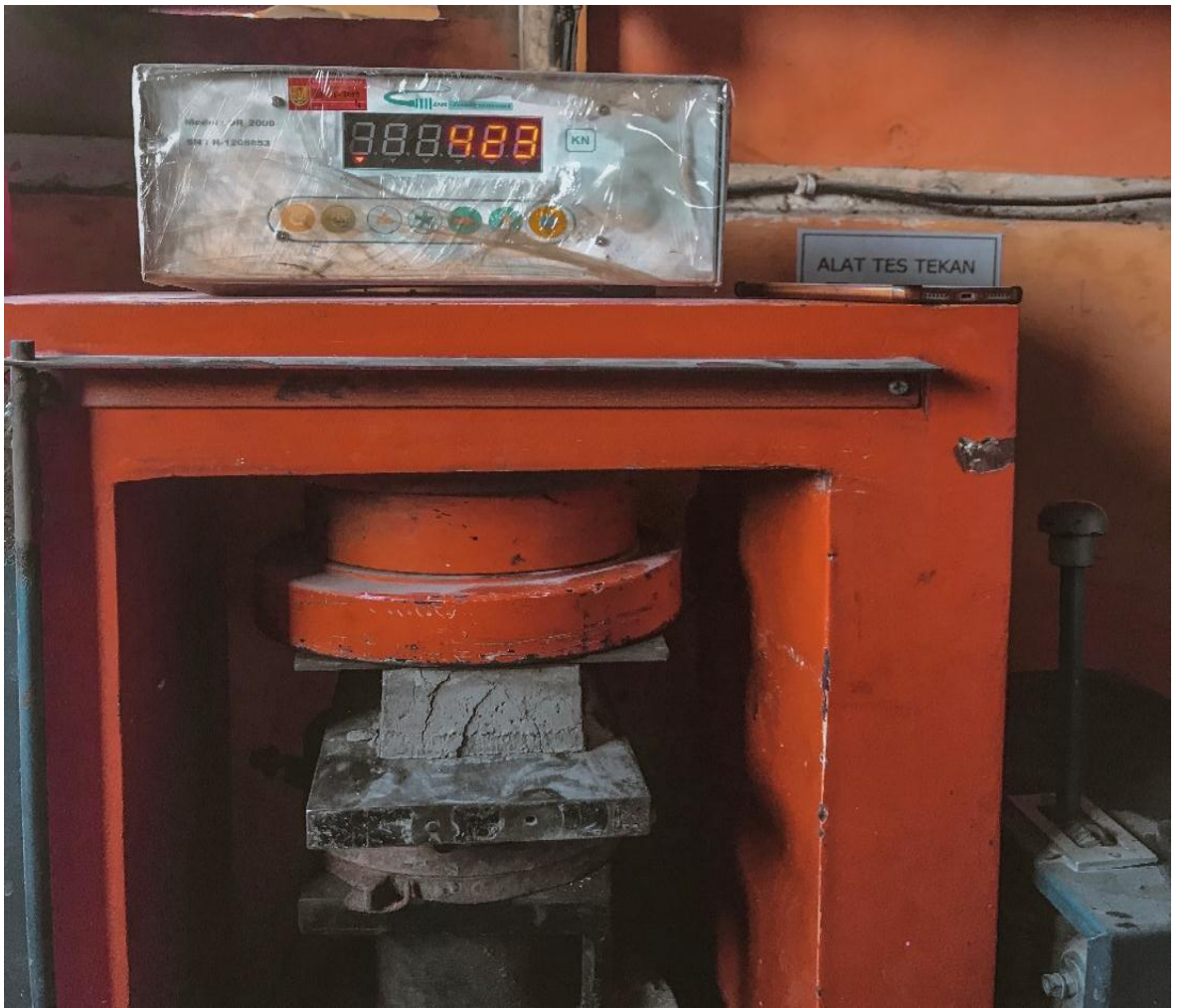
Gambar 18. Uji Tekan Paving Block ( Laboratorium PT.Ava Beton)
