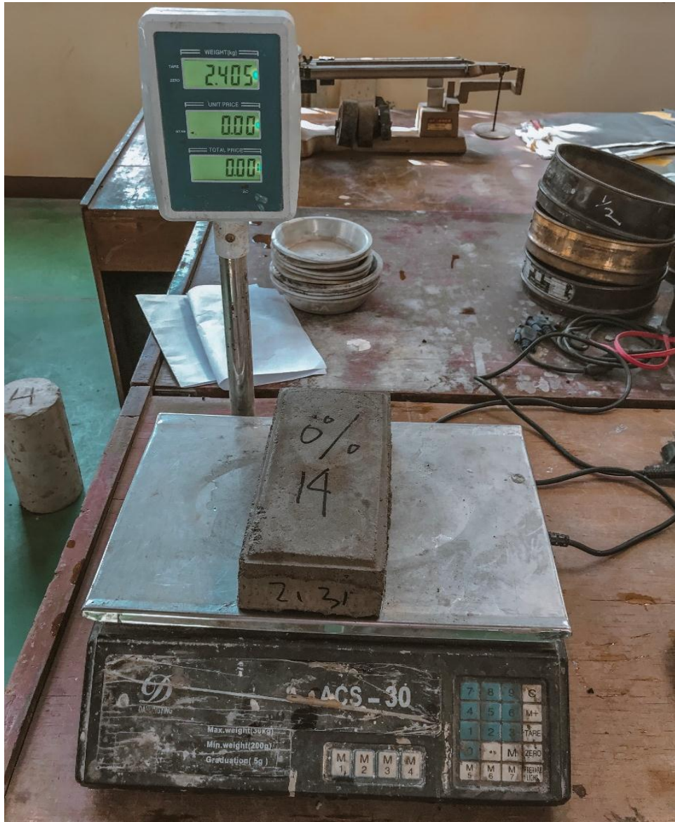
Gambar 14. Penimbangan paving block
