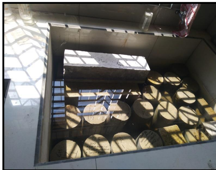
Perawatan beton didalam bak perendaman
