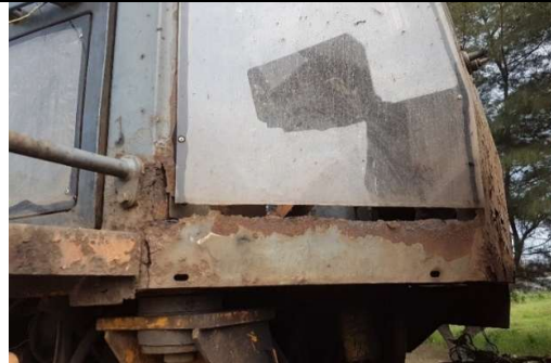
Wheel Loader 835 kabin keropos
