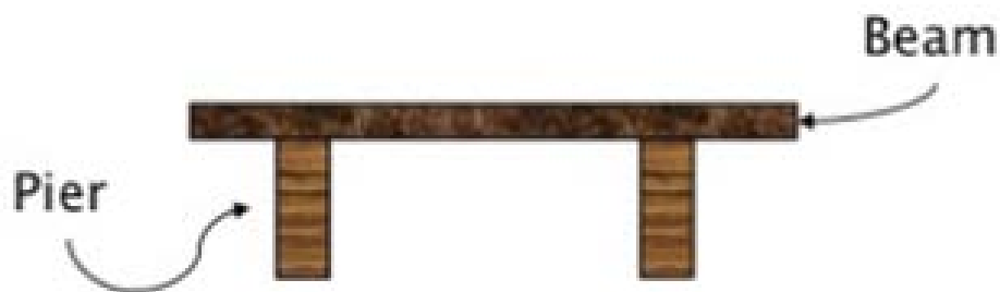
Figure 1.1. Simple bridge beam, a basic concept of the bridge.
