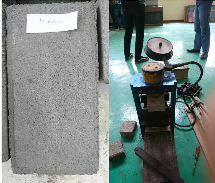
Gambar 11. Uji Kuat Lentur Cone Block Normal
