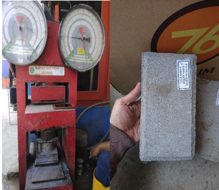
Gambar 1. Uji Kuat Tekan Cone Block Normal
