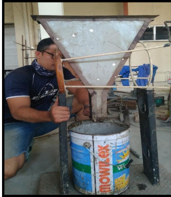
Gambar 7.1 (V Funnel Test)
