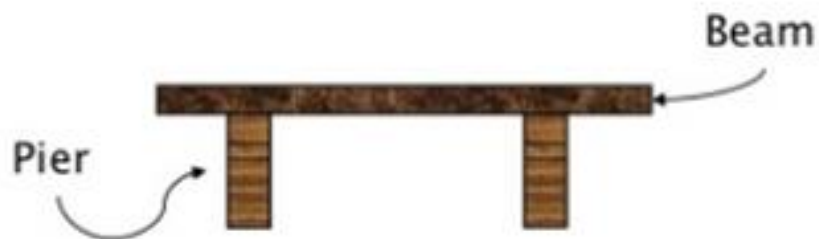
Figure 1.1. Basic concept of simple bridge
