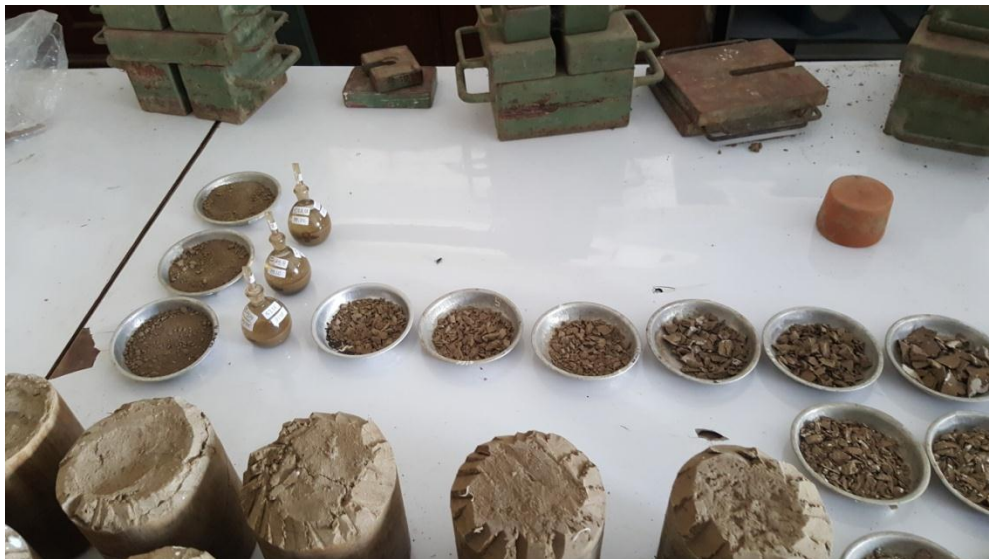
Pengujian Kadar Air, Berat Jenis
